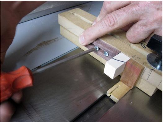
**Loosen** the guide screws and place the block between the guides.
